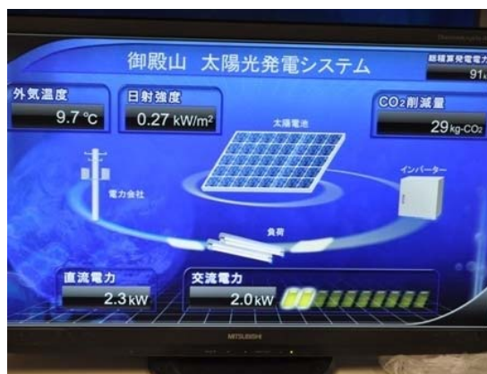
GDC Gotenyama: Solar power generation monitor
